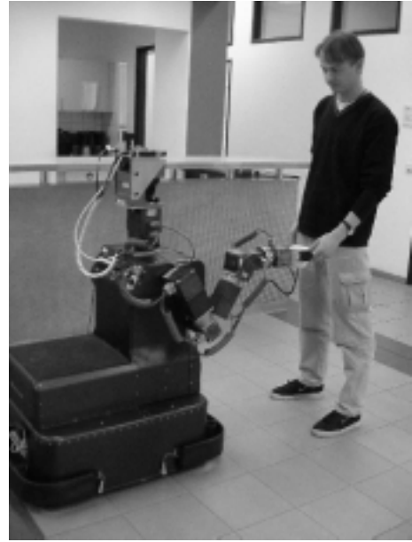
Figure 9: Scenes from the coffee serving scenario: the cup of coffee is handed over to the thirsty scientist. When doing this, the robot monitors the wrist forces and waits until the person has taken hold of the cup.
