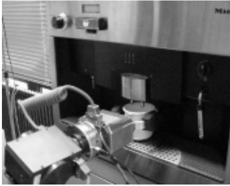
Figure 7: Scenes from the coffee serving scenario: the robot drives to the coffee maker and inserts the cup in the coffee dispenser.
