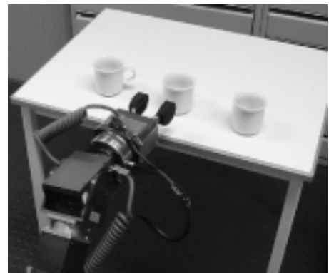
Figure 6: Scenes from the coffee serving scenario: after docking by the table the robot locates a cup and picks it up.
