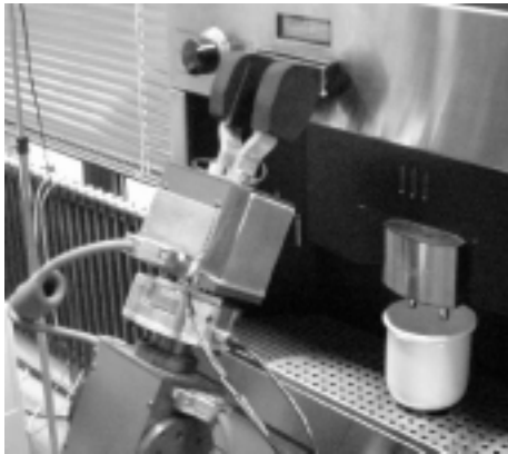
Figure 8: Scenes from the coffee serving scenario: the robot presses the button on the coffee maker.
