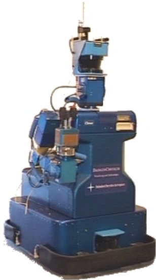
Figure 4: The robot “Clever” used in the experiments. The robot consists of a differential drive platform equipped with a 7-DOF Amtec manipulator and a Sick lidar plus a set of colour CCD cameras mounted on a pan/tilt unit. The arm is equipped with a force-torque sensor between the wrist and the gripper, which is a standard parallel jaw gripper with force sensors in the “fingers”.
