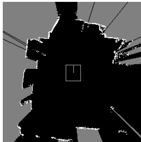
Figure 1: Evidence grid used as virtual joystick. White denotes occupied space, black freespace, and grey unknown. In the plot, the robot is standing in a room with a doorway approximately 2.5 meters in front of it.
