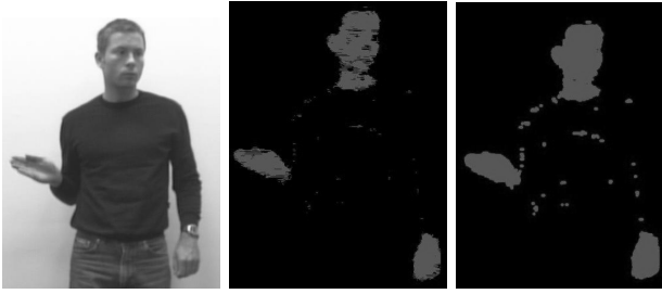
Figure 2: Image Processing Steps (Grabbed image, Color Segmentation, Closing Operation).
