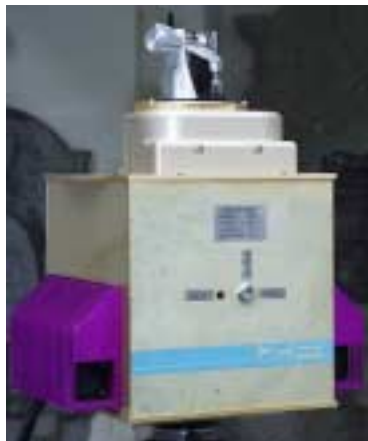
Fig. 1: Imaging Z+F Laser Radar
