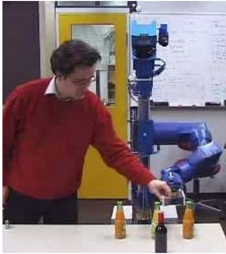
Figure 3: A mobile manipulator receiving tactile help in an ambiguous situation.
