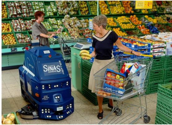
Figure 1: An autonomous cleaning robot based on the Siemens navigation system SINAS.
