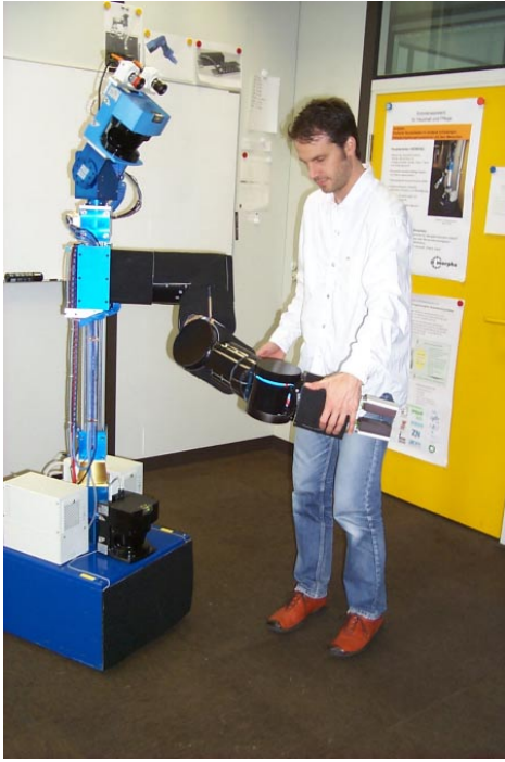
Figure 2: A mobile manipulator engaged in tactile interaction through its sensitive artificial skin.
