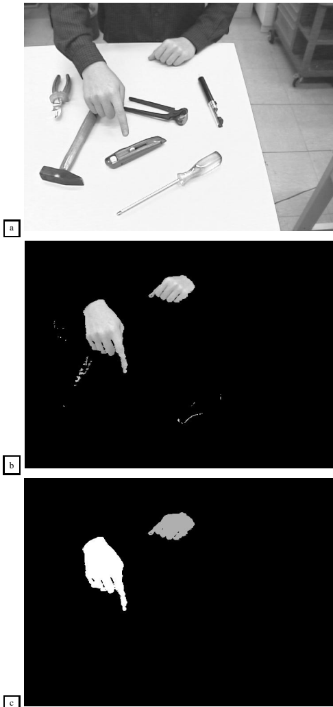
Figure 3: Figure (a) shows a typical situation during a man machine interaction. By using the color samples, acquired during the calibration phase, we get all regions, which possibly are skin areas (figure (b)). Finally we check the median disparity of adequate big clusters, to get the pointing hand, which should be the nearest cluster to the camera (figure (c)).
