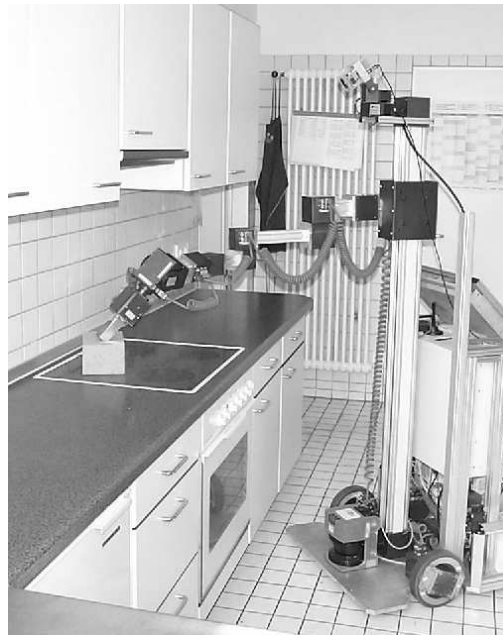
Figure 1: Mobile Manipulator for home environments.
