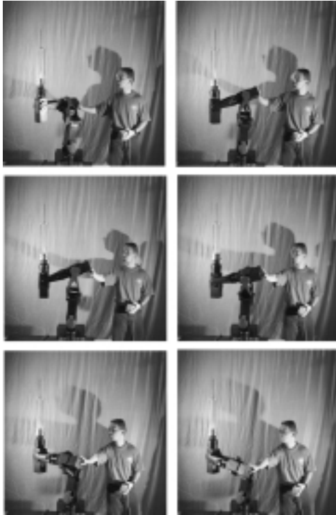
Figure 8. Nullspace motion by touch through sensing external joint torques \tau_{ext} applied by the user. Note: A human subject would seldomly succeed to balance a rod while somebody touches his elbow.
