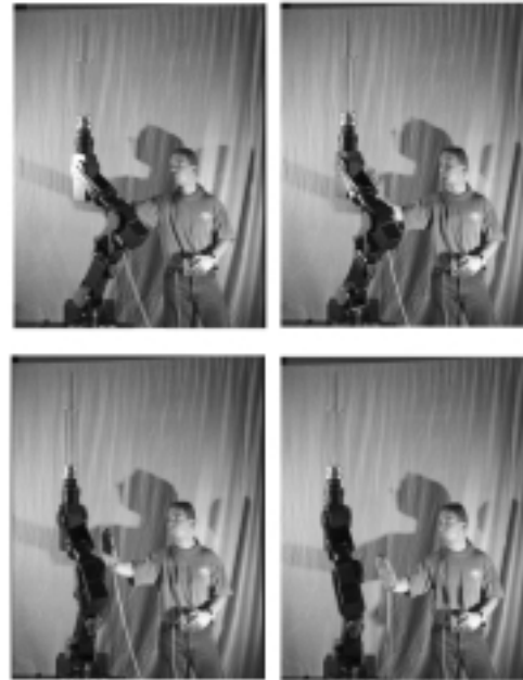
Figure 9. Collision avoidance with nullspace motion, the colliding object is represented by the data glove with position tracker in the user’s right hand.
