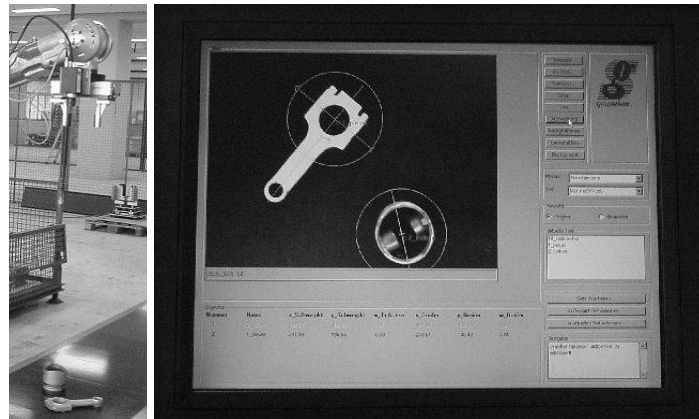
Figure 6: Manufacturing Assistant: learning objects. Left the scene with the manipulator looking down on the conveyor belt with the objects. Right the GUI used to teach the objects.
