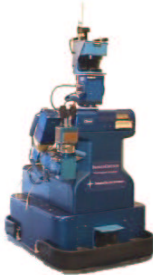
Fig. 2. The robot “Clever” used in the experiments. The robot consists of a differential drive platform equipped with a 7-DOF Amtec manipulator and a Sick lidar plus a set of colour CCD cameras mounted on a pan/tilt unit. The arm is equipped with a force/torque sensor between the wrist and the gripper, which is a standard parallel jaw gripper with force sensors in the “fingers”.
