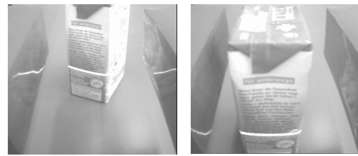
Figure 7: The view from the gripper camera at the beginning and endpoint of the grasping motion.
