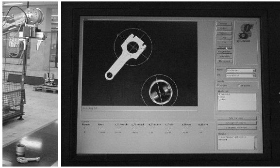
Figure 4: Learning objects. Left the scene with the manipulator looking down on the conveyer belt with the objects. Right the GUI used to teach the objects.
