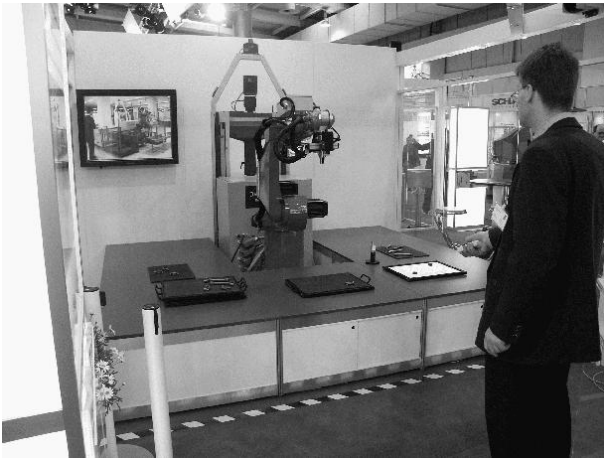
Figure 2: The setup for the order-picking demonstrator shown at the Hannover Fair 2002. The operator is showing with the laser pointer where the robot should place the next item. The items are retrieved from the storage areas left and right to the robot. The striped line in the floor marks the border which, when unexpectedly crossed, will cause the robot to come to an emergency stop. This is ensured by the Sick PLS laser scanner partly visible in the upper right corner of the image.
