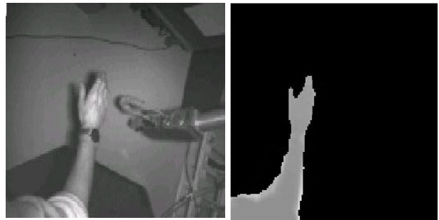
Figure 13. Range image and corresponding segmented range image with obstacle.
